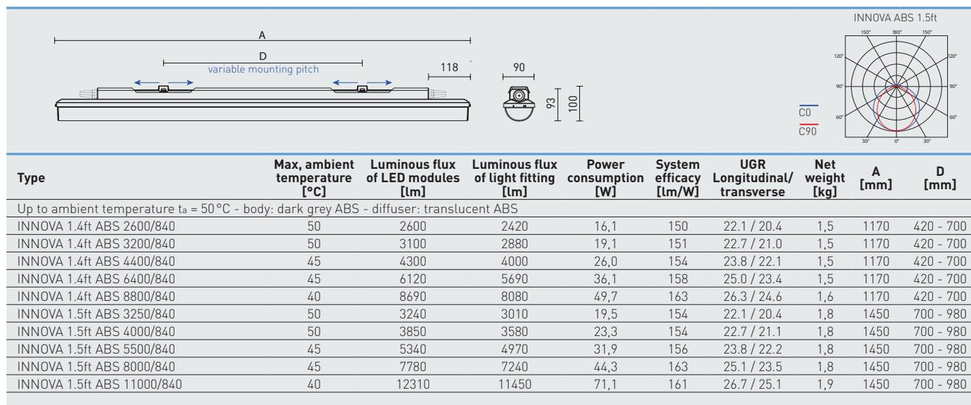
INNOVA 1.4ft ABS 3200/840 = suitable replacement for tube light fitting PRIMA 136 ABS – 1 × 36 W
